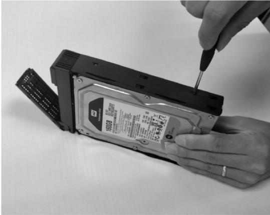
3.5" hard drive(4screws fixed on both sides)
