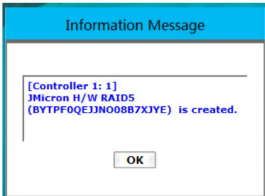
7. HDDs or HDD group that has been set RAID mode will be displayed on computer later and it can be started to use after initiating and partitioned formatting. (Please try to restart the HDD enclosure and computer or reset RAID mode if the formatting of HDDs or HDD group is fail.)
