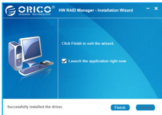
3. The shortcut of ORICO HW RAID Manager software will appear on PC desktop after finishing the installation. Please turn on the power of the HDD enclosure and HDD, double click to run the software to set or manage RAID.
